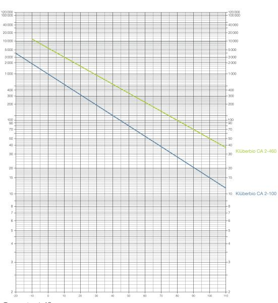
Kinematic viscosity in mm<sup>2</sup>/s
